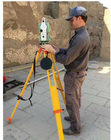
Owen using total station for photogrammetric recording of wall reliefs, Luxor Temple, November 7, 2018. Photo: Ray Johnson.
